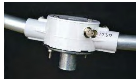
PHOTO 4: The feedpoint of the loop antenna.
