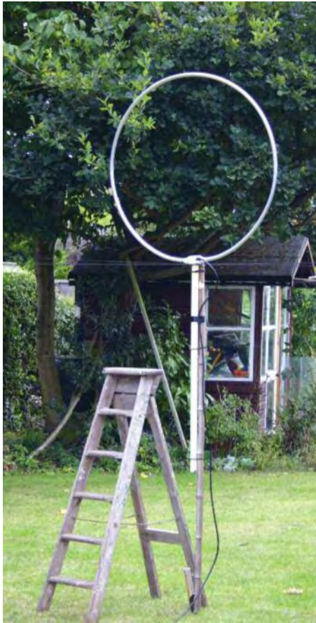
PHOTO 1: The ALA1530 under test at G3MPN.
